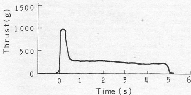
Figure 3. Thrust-time curve for a hollowed burning surface.
